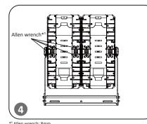
\*1 Allen wrench: 8mm \*2 Minimum M12 screws (Not provided) \*3 Screw nuts (Not provided)
